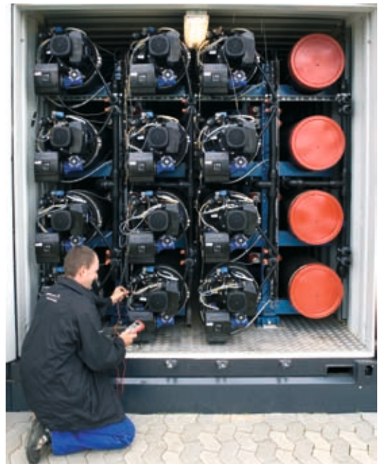
The pre-treatment container consists of 12 PBR reactors and allocated space for additional reactors, which can be added when the need for extra capacity arises.
